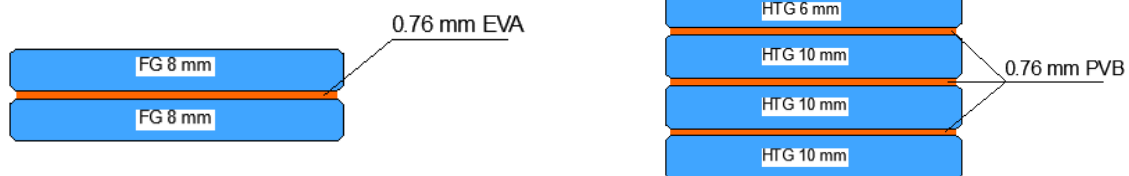
Fig. 5: Cross section examples of double and multi laminated glass panel
