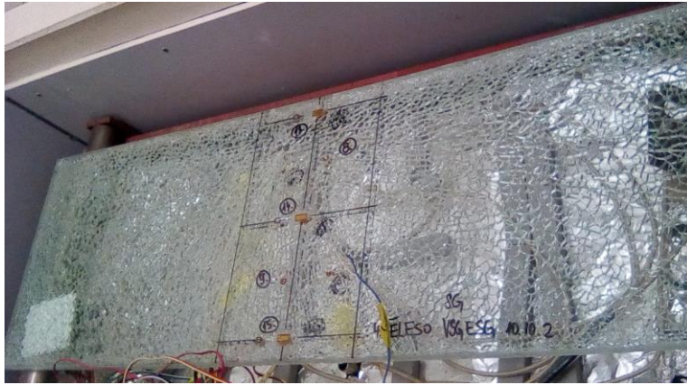
a) Abrupt collapse during the test
