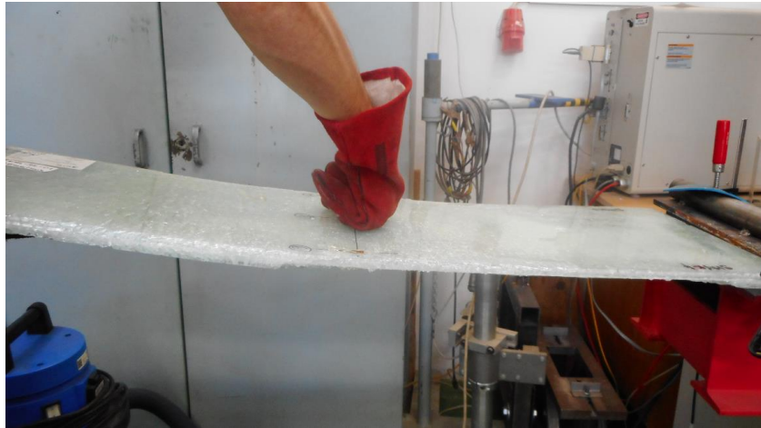
c) SG 5000: specimen stayed on the support being stiff enough to carry itself and added arm load
