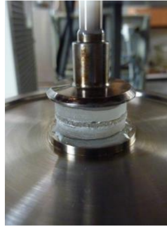
b) DMTA in torsion mode, rheometer [70]
