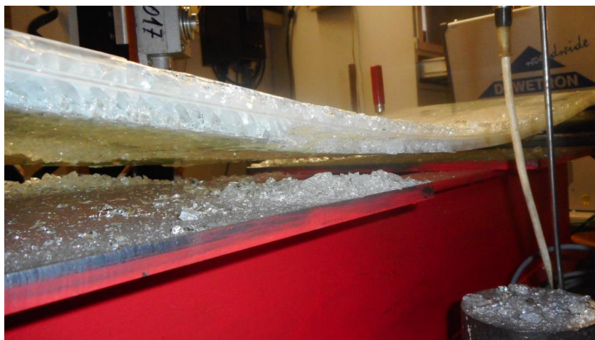
b) EVA L: specimen fell down the support with massive transverse crack over the specimen
