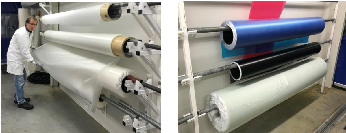
Fig. 64: Storage of interlayers in big roles before lamination
