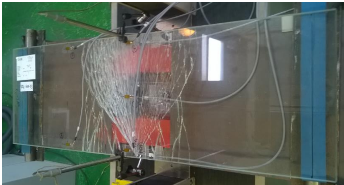
a) Testing specimen made of FG laminated with Trosifol BG, shards are adhered to the interlayer
