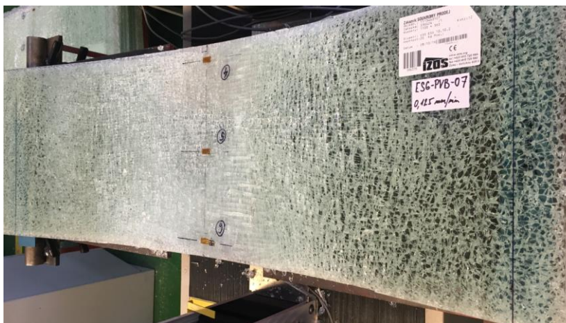
a) Trosifol BG: specimens fell down the support, no transverse cracks are present
