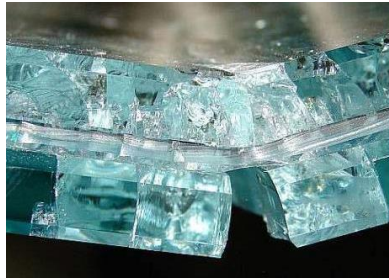
Fig. 8: Shards adhered to the interlayer after failure of LG panel in bending [1]
