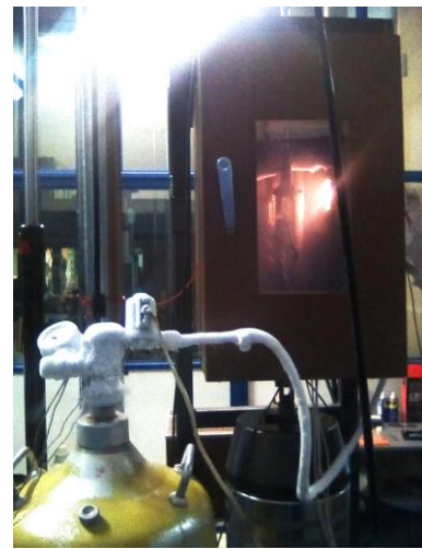
b) Specimen in the climatic chamber and Dewar vessel with nitrogen
