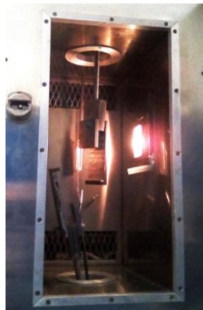
c) Climatic chamber with metal jaws
