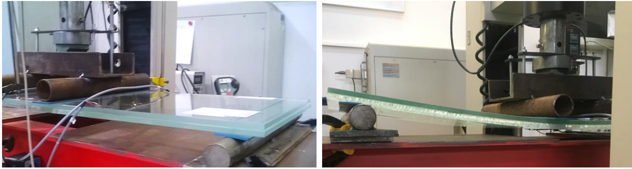
a) FG right before total failure, no warning effects given by deflection
