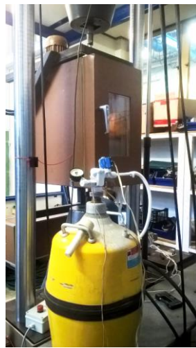
b) Specimen in the climatic chamber and Dewar vessel with nitrogen
