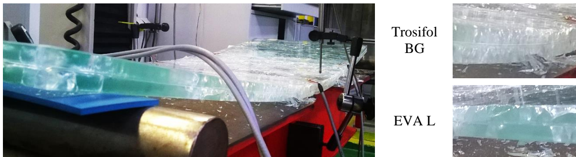
b) Heat strengthened glass (HSG), specimen still on the support after total failure
