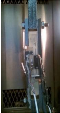
a) DMTA in single-lap shear mode, MTS
