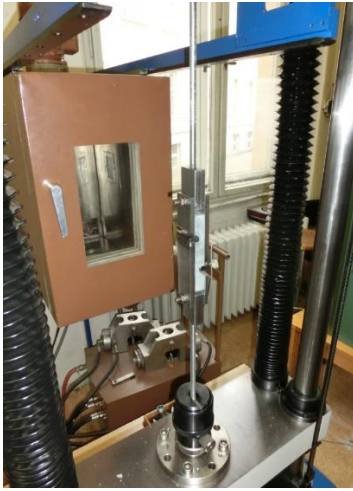
a) Testing frame of single-lap shear tests
