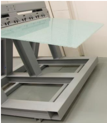
a) LG panel with polyethylene-co-methacrylid acid ionomer interlayer
