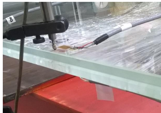
a) Testing specimen made of FG laminated with Trosifol BG, shards are adhered to the interlayer
