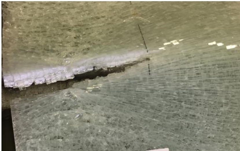
b) EVA L: specimen fell down the support with massive transverse crack over the specimen
