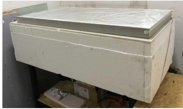
h) Closed climatic chamber for creep tests ensures climatic conditions, test is running
