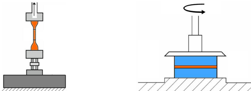
a) Tensile tests of a raw interlayer in hydraulic machine [27]
