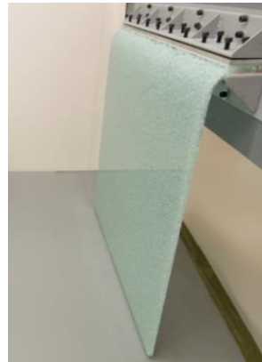
b) LG panel with polyvinyl butyral interlayer
