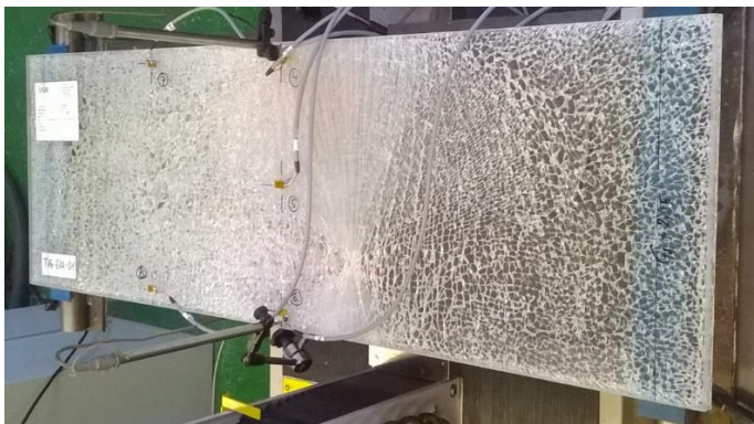
b) Testing specimen made of HTG laminated with EVA L, shards are adhered to the interlayer
