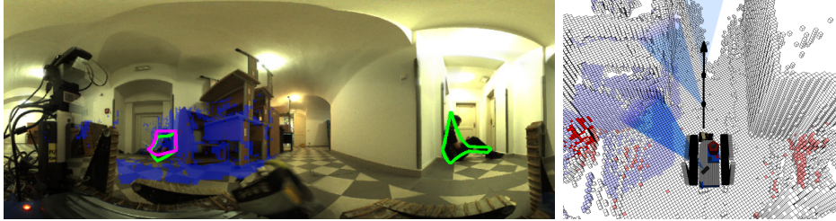
Figure 3.7: Left: Panoramic RGB image with segmented humans outlined by green (RGBD data segmentation) and magenta (RGBDT data segmentation) contours. The reprojected thermal measurements collected up to the current time are emphasized by blue overlay. Right: Reconstructed and segmented voxel map with accumulated thermal measurements displayed in blue color. Light red denotes the voxels marked as corresponding to human based on RGBD data only, dark red denotes the voxels marked as human based on the data with additional temperature measurements. Robot path with positions is denoted by black arrow with dots and selected thermal viewpoints are outlined by blue cones. The thermal camera is controlled to maximize the long-term sum of \Delta \mathcal{H} .
