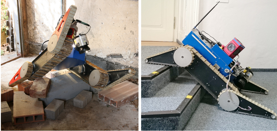
Figure 4.1: Tradr UGV. Track flippers visible on the side of the robot. A policy governs active tilting of the flippers assuring a safe traversal .
