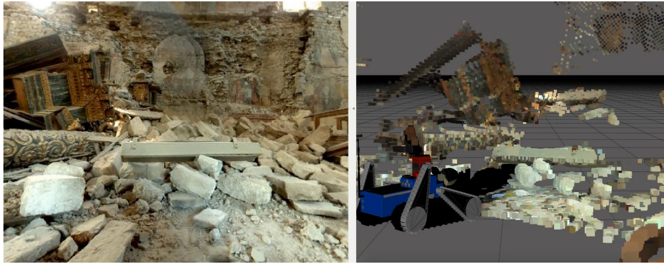
Figure 1.1: Example of search-and-rescue environment. Damaged church after the earthquake in Amatrice in Italy 2016. Left: RGB image captured by onboard cameras. Right: colored pointcloud obtained using rotational Sick LiDAR.
