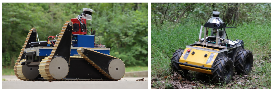
Figure 5.5: Left: Upgraded tracked Tradr UGV. Right: Husky A200 wheeled robot.
