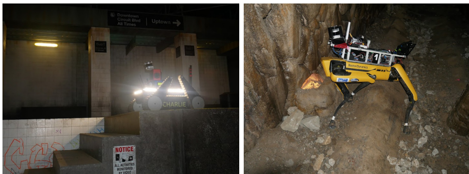
Figure 5.1: Left: Tradr UGV in the simulated metro station. Right: Boston Dynamics Spot robot in cave.
