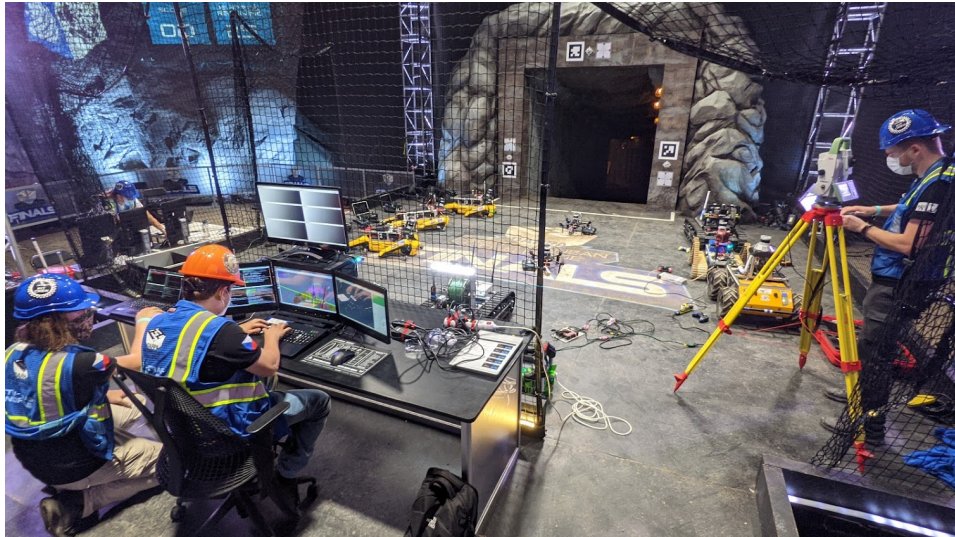
Figure 5.3: Staging area at finals during the preparation for the scored run. Robots are already on their place. Their exact position is measured by the person at right side of the image. Base station is prepared by the team operator (the person with orange helmet).
