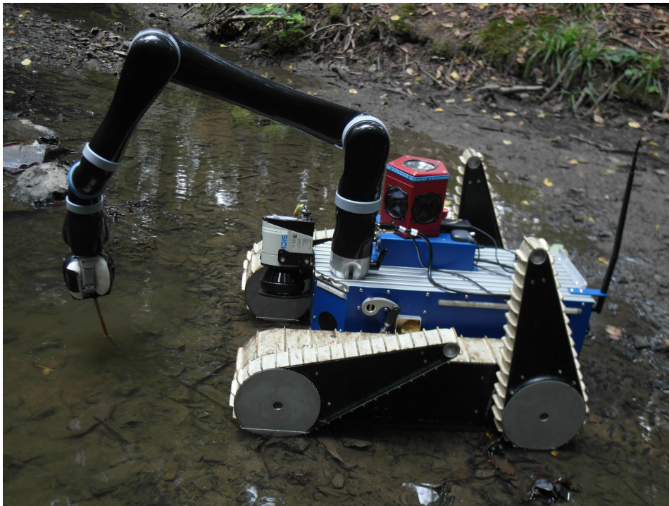
Figure 2.6: Search-and-rescue UGV developed as part of the TRADR projects, equipped with a Point Grey Ladybug 3 omni-directional camera, a rotating SICK LMS-151 laser range finder and a Kinova Jaco robotic arm, in our case used for contact exploration of terrain with a wooden stick tool.
