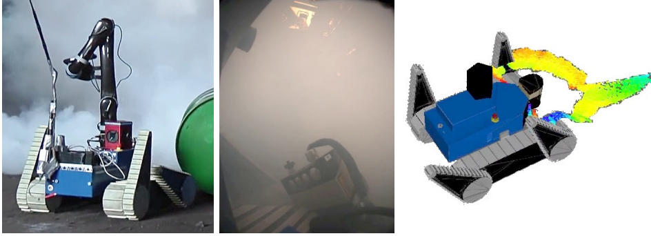
Figure 2.7: Left: UGV robot approaches smoke area. Middle: Example of visual information that the operator sees inside a cloud of smoke. Right: Output of the laser range-finder (rainbow-colored point cloud in the right half of the image). Laser beams are randomly reflected by smoke particles. The resulting 3D point cloud is just noise close to the robot.
