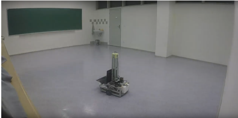
Figure 5.32: Example of the procedure of measurement of illuminance using the second robotic unit.
