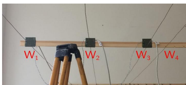
Figure 2. A photo of the measurement setup with W_4 at a distance of 10 cm from W_3 . [30]
