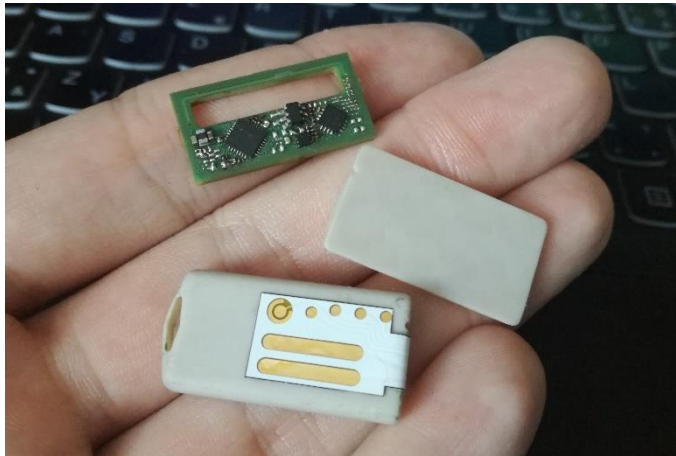
Figure 6: PEEK enclosure and PCB
