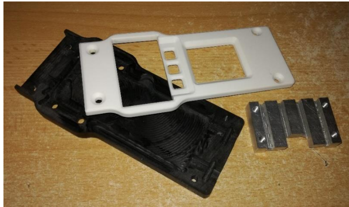
Figure 10: Plastic enclosure for the lower portion of charger device
